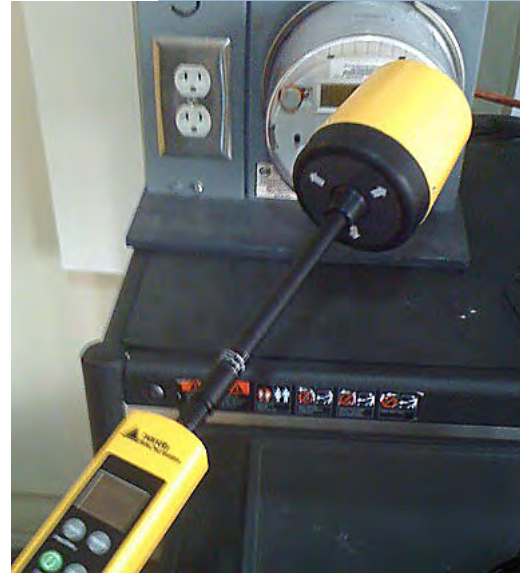
Radio frequency reader measuring smart meter radio frequency levels during briefing for Assembly Member Huffman.
